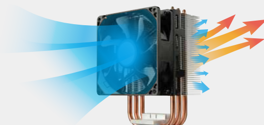
Others - Cooling air leaks from sides
