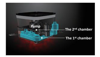
Patented Dual-Chamber Design water block Patented Dual-Chamber Design isolate the pump from the heat to prolong the cooler's lifetime
