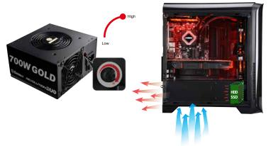
Application 2: For normal/open PC case REVOLUTION DUO can also improves the system cooling when FMA is set at high.
