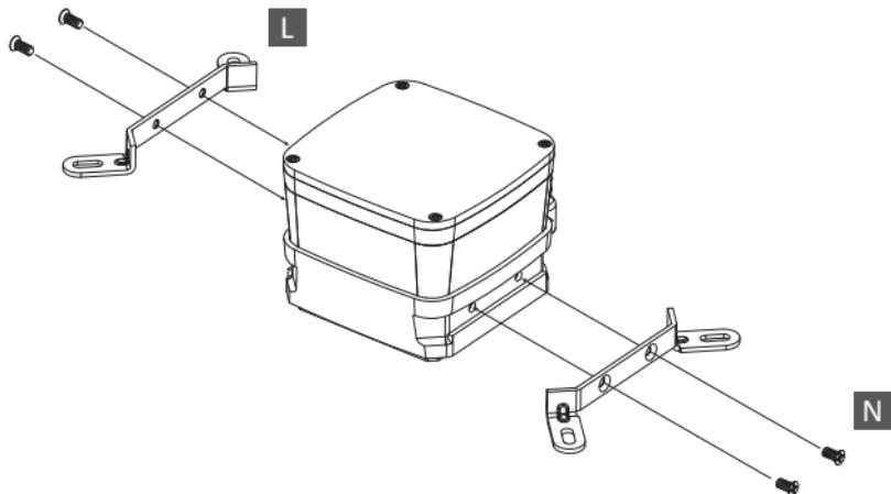
**EN** Install the Intel clip to the pump.
