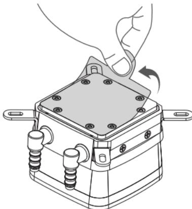
**EN** Remove the protect film from the cold-plate.
