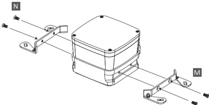
**EN** Install the AMD clip to the pump.
