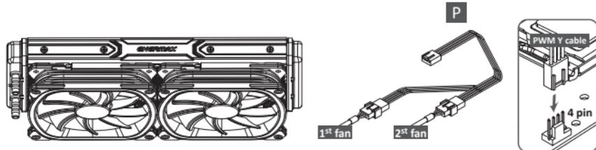
**EN** Connect the fan connector to the motherboard.
