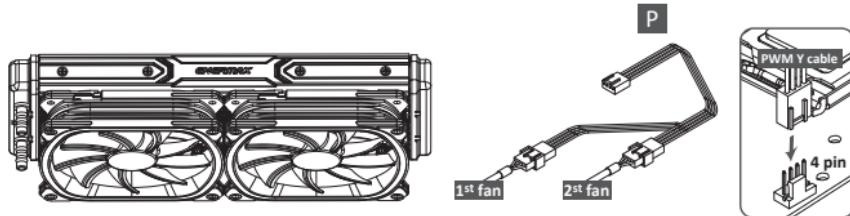
**EN** Connect the fan connector to the motherboard.
