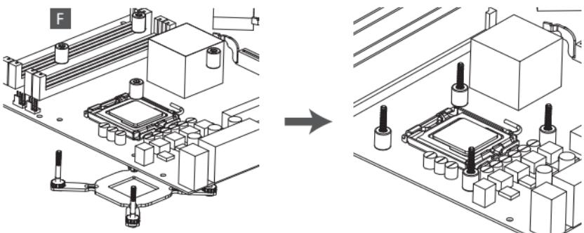
**EN** Install the Intel back plate on to the back of motherboard; fix the back plate with the stand-off.
