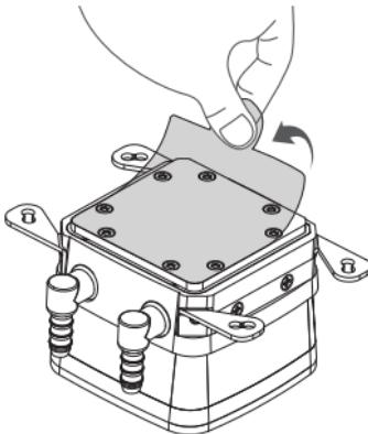
**EN** Remove the protect film from the cold-plate.
