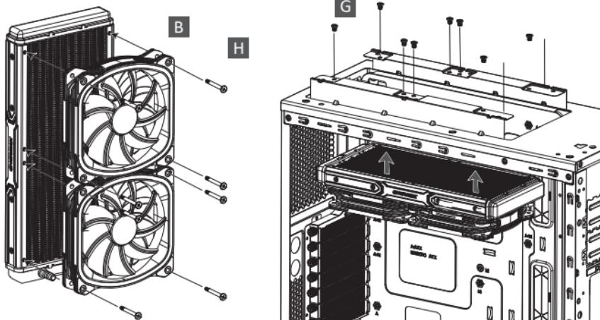
**EN** Attach the fan and the radiator to the chassis.
