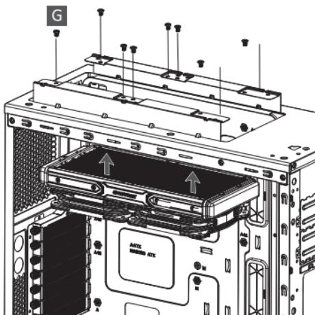
**EN** Attach the fan and the radiator to the chassis.
