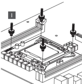
**EN** Tighten the Intel LGA2011/2011-3/2066 screw to the motherboard.
