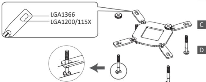
**EN** Insert the position screws into the proper holes on the back plate. Then use the washers to fix the position screws.
