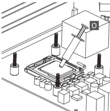
**EN** Apply the thermal grease evenly on the CPU surface..
