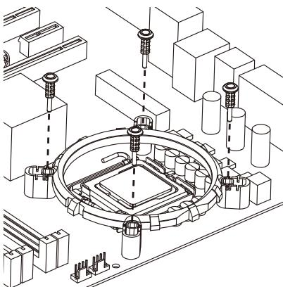
**EN** Press the push-pins into the clips and ensure the Intel mounting bracket is safely installed on the motherboard.
