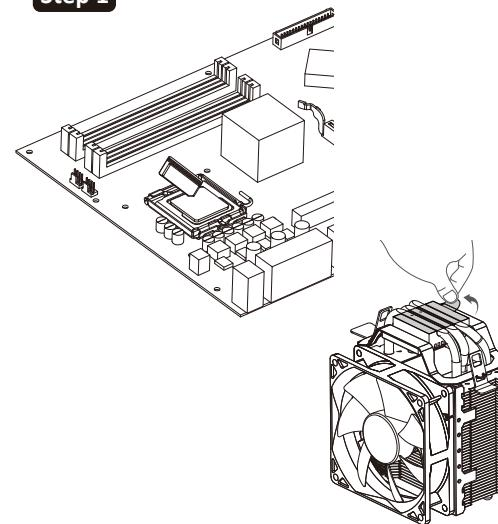
EN Apply the thermal grease evenly onto the CPU surface. Remove the protective film from the cooler base. (If your CPU platform is AMD, please skip to step 4-2)
