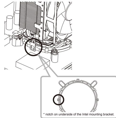
**EN** Place the cooler on the CPU. Clasp the hooks of AMD mounting bracket on to the notch on underside of the Intel mounting bracket as illustrated.
