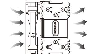
**EN** Connect the fan 4 pin header to the CPU fan power socket on the motherboard.
