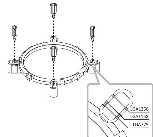
EN Insert the clips into the proper holes on the Intel mounting bracket.
