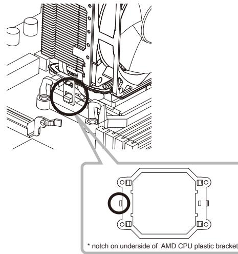
**EN** Place the cooler on the CPU. Clasp the hooks of AMD mounting bracket on to the plastic notches at the top end of the AMD CPU socket as illustrated.
